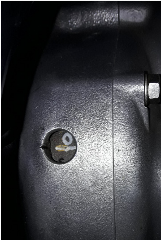
Picture 4 – Setting the Advance of ignition spark by setting the Trigger tooth position
